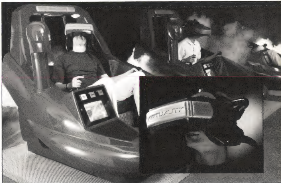
The arcade 'sit-down modules'. Inset: The 'Visette' visor generates an internal 3D display on LCD screens.
